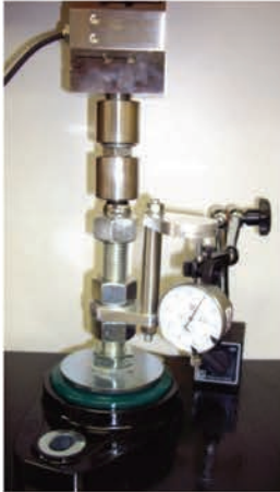
1. Axial Load Test [Vertical down direction]
