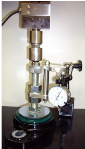
1. Axial Load Test [Vertical down direction]
